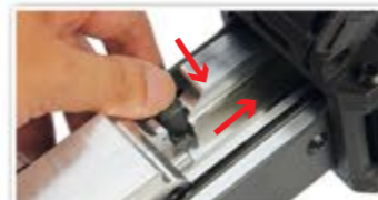
Open the feed tray cover, press the hop up release button.
