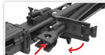
Insert the barrel then close the flap.
